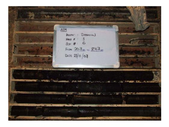
Figure 2-22: Cored Borehole from the Current Drilling Programme, Doshin Coal Deposit, December, 2007
