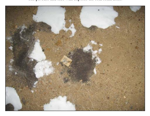
Figure 5-13: Chips (cuttings) from the Previous Drilling Programme in Khashaat Area
